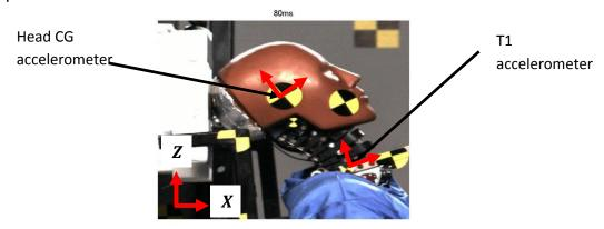
At 80ms, the following two accelerometer readings were observed (in SI units):
